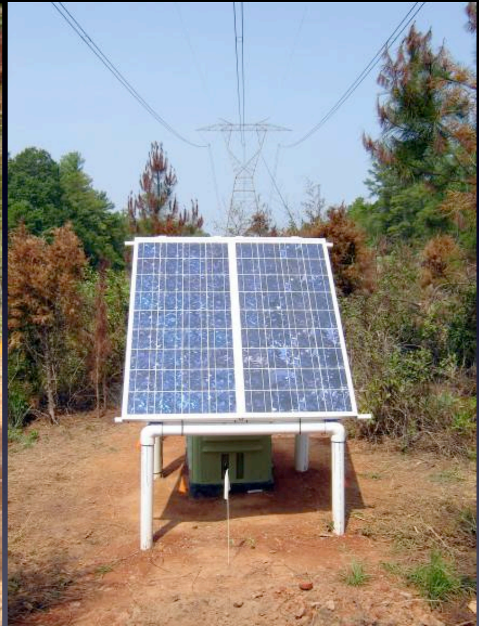
Solar panel and prototype electronics package
